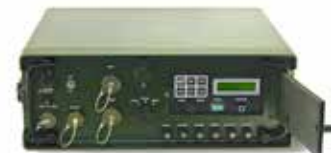
DSD 72A-SP military bulk data encryption system.
