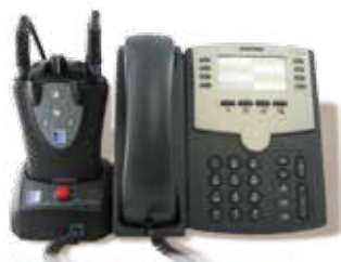
HSE 6000 headset radio encryptor enables secure commander's conferencing.
